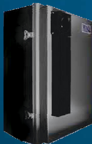
Processor Dimensions H 60.96cm (24") W 39.37cm (15.5") D 20.035cm (10.25")
